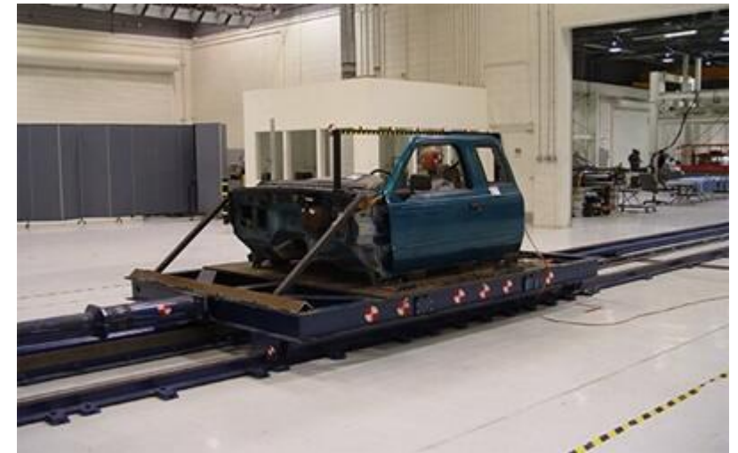
Catapult – Crash Test Sled Repeatable and reliable impact conditions
